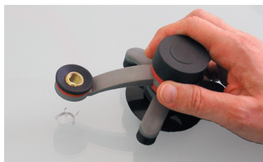
2. the roger's tool holder is fixed above the damaged spot, ...
